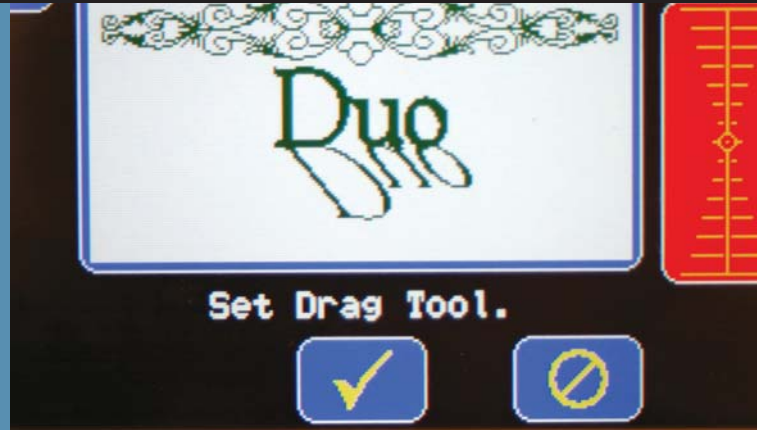
(left) Preview laser raster and diamond drag portions of a job via the color touch screen before you engrave (below) Diamond Drag on Medallions, reflective metals
