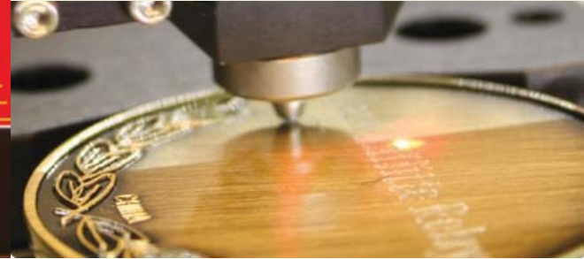
(left) Preview laser raster and diamond drag portions of a job via the color touch screen before you engrave (below) Diamond Drag on Medallions, reflective metals
